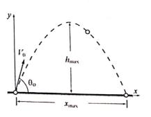
Consider the case where  $V_0 = 600 \text{ ft/s}$  and  $\theta = 54^\circ$ . Define  $V_0$  and  $\theta$  as MATLAB variables and calculate  $t_{travel}$ ,  $x_{max}$ , and  $h_{max}$  ( $g = 32.2 \text{ ft/s}^2$ ).
