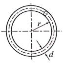
anonymous function that calculates the weight of the coating. The function should have four input arguments, r, d, t, and  $\gamma$ . Use the anonymous function to calculate the weight of a gold coating ( $\gamma = 0.696 \text{ lb/in.}^3$ ) of a ring with r = 0.35 in., d = 0.12 in., and t = 0.002 in.
