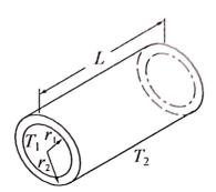
and an inner radius of  $r_1 = 3$  cm. The external temperature is  $T_2 = 20$ °C and the internal temperature is  $T_1 = 100$ °C.
